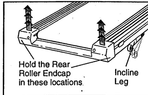
To lower the back end, first raise it past the highest position, and then lower it. **CAUTION:** Before exercising, push on the back of the treadmill to make sure that the incline legs are locked in position. Do not place objects under the treadmill to change the incline; change the incline only as described above.
