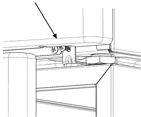
**NOTE:** If front mounting holes are not present on the washer base, drill them out with a 5/32" drill bit, or order an installation kit part number 134504100.
