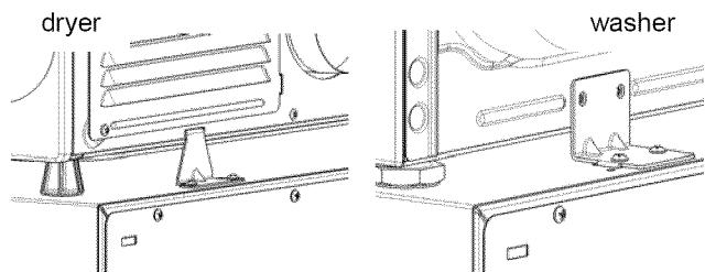
**NOTE:** If slots or mounting holes do not align, make sure the washer or dryer leveling legs are adjusted fully into the unit. Turn each leg tight to the base.
