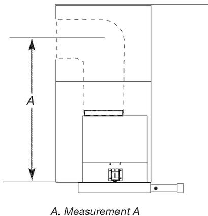
Transfer measurement A to the cabinet back wall. Measure from the underside of the cabinet or wood filler strips, if used. Mark the cutout as shown. Use a saber saw or keyhole saw to cut a round opening for the vent.
