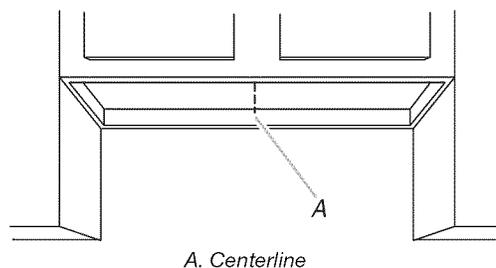
2. Measure and mark lines as shown for your size of range hood. Use a saber saw or keyhole saw to cut an opening through the underside of the cabinet.
