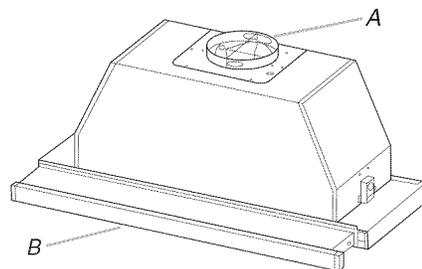
A. Clapet anti-reflux
