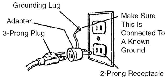
**Figure 3 - 2-Prong Receptacle with Adapter**
