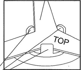
The pins of the turntable motor shaft
