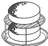
**Low rack (Broiling trivet)**—for convection, broiling or high mix.
