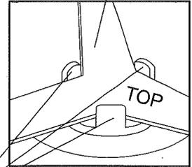
The pins of the turntable motor shaft
