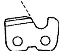
Backslope in side plate— caused by holding sharpener too high. Chain won't feed properly; cutters wear fast at heel
