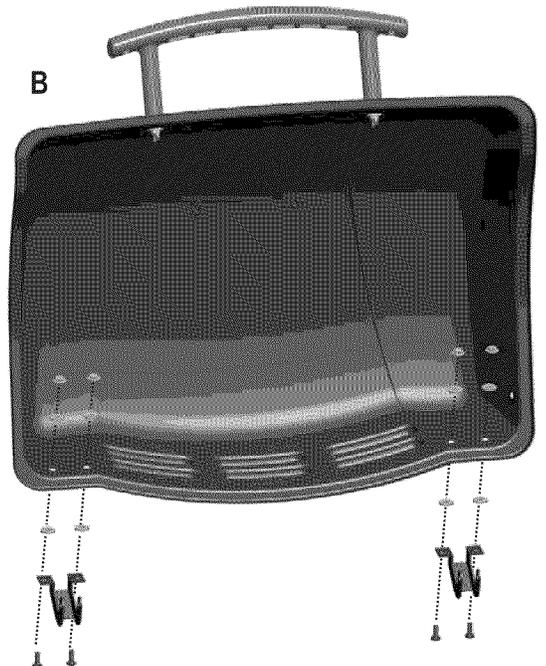
**14** Place lid assembly onto firebox, aligning hinges. Hinges on lid fit inside hinges on firebox. Secure using **two hinge pins** and **hitch pins**.
