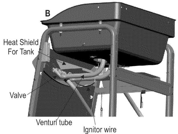
**Make sure the Venturi tubes are located underneath Heat Shield**
