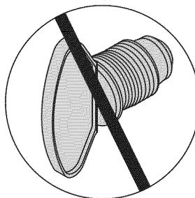
**Do not use a POL transport plug (plastic part with external threads)! It will defeat the safety feature of the valve.**
