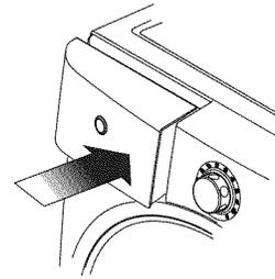
Insert liquid cup when using liquid detergent.
