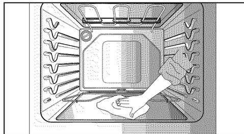
The bake element is designed to be tilted up using your hand from the front of bake element. This will allow easier access to the oven bottom for cleaning. Be careful not to raise the element more than 4 or 5 inches from the resting position.
