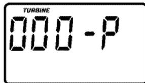
The letter (P) and dash or dashes indicate position switch operation. The letter shows if the switch is closed. A dash shows when the switch is open.
