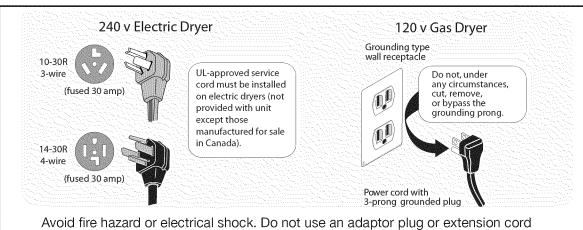
or remove grounding prong from electrical power cord. Failure to follow this warning can cause serious injury, fire or death.
