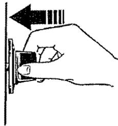
Push in and turn the lower oven drawer knob to any desired setting
