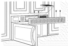
To install a new filter, remove plastic and other outer wrapping from the new filter.
