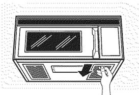
**To remove**, slide them to the side using the tab. Pull them down and out.
