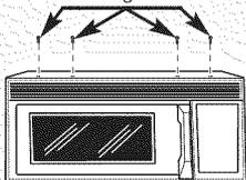
To remove the charcoal filter, disconnect power at the main fuse or circuit breaker panel or pull the plug.
