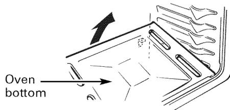
4. Locate the pilot in the back of the oven bottom. The pilot is attached to the left side of the oven burner.
