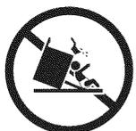
To reduce the risk of tipping the range, the range must be secured by a properly installed anti-tip bracket. See installation instructions shipped with the bracket for complete details before attempting to install.
