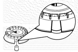
Replace the matching size caps onto the heads. There is one small, two medium and one large cap. Sizes are stamped into the bottom of the caps.
