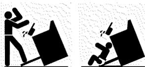
**▲ WARNING:** If your range is removed for cleaning, servicing or any reason, be sure the anti-tip device is re-engaged properly when the range is replaced. Failure to take this precaution could result in tipping of the range and cause injury.
