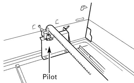
5. To light the oven pilot, push in and hold the oven control knob while lighting the pilot with a long match or match holder. Once the oven pilot is lit, continue holding the oven control knob for one minute before releasing.
