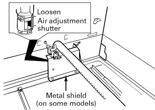
On some models, remove the metal shield at the rear of the cavity.
