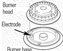
Make sure the hole in the burner head is positioned over the electrode and that the burner head is fully inserted inside the burner base. A small gap between the base and head is normal.
