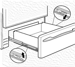
**NOTE:** For models with an electric warming drawer, before performing any adjustments, cleaning or service, disconnect the range electrical power supply at the household distribution panel by removing the fuse or switching off the circuit breaker. Make sure the warming drawer heating element is cool.
