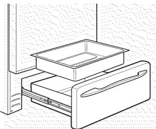
**NOTE:** For models with an electric warming drawer or lower oven drawer, before performing any adjustments, cleaning or service, disconnect the range electrical power supply at the household distribution panel by removing the fuse or switching off the circuit breaker. Make sure the drawer heating element is cool.
