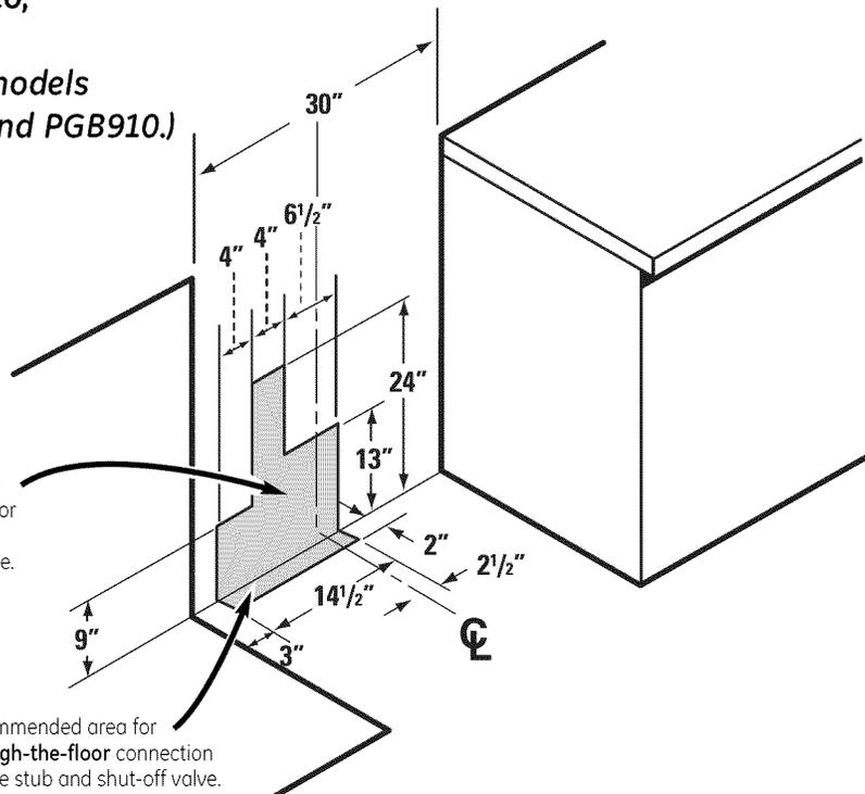
Recommended area for through-the-floor connection of pipe stub and shut-off valve.
