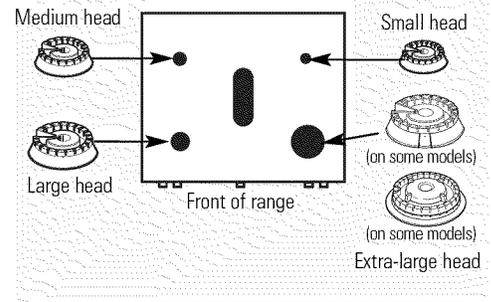
Make sure the slot or hole (depending on model) in the burner head is positioned over the electrode.
