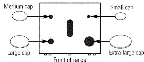
Make sure that the heads (on some models) and caps are replaced in the correct locations.
