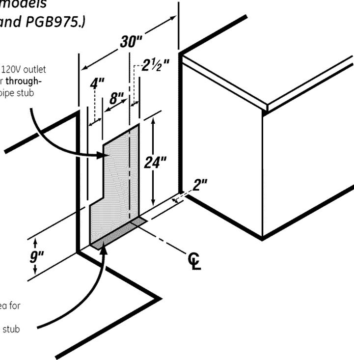
Recommended area for through-the-floor connection of pipe stub and shut-off valve.
