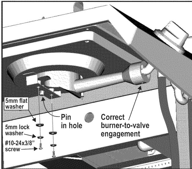
Valve should be in center hole in burner tube.
