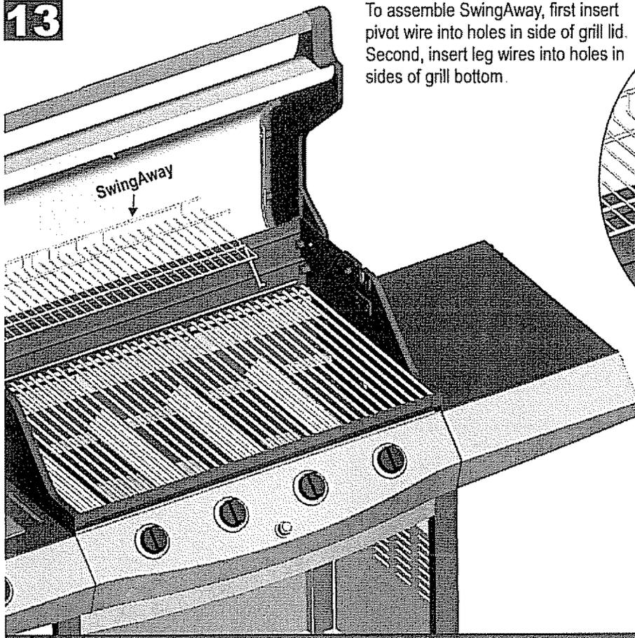
To assemble SwingAway, first insert pivot wire into holes in side of grill lid. Second, insert leg wires into holes in sides of grill bottom.
