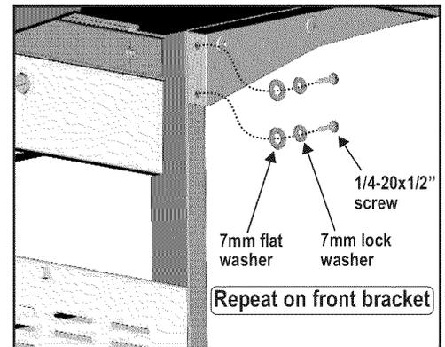
**7** Place sideburner shelf over left cart legs. Lip of shelf should fit between grill bottom and leg brace. Secure shelf brackets to cart legs using two **1/4-20x1/2"** screws, **7mm** lock washers and **7mm** flat washers. **Fully tighten screws inside grill bottom and at back of grill at this time. Refer to Steps 4 and 5.**
