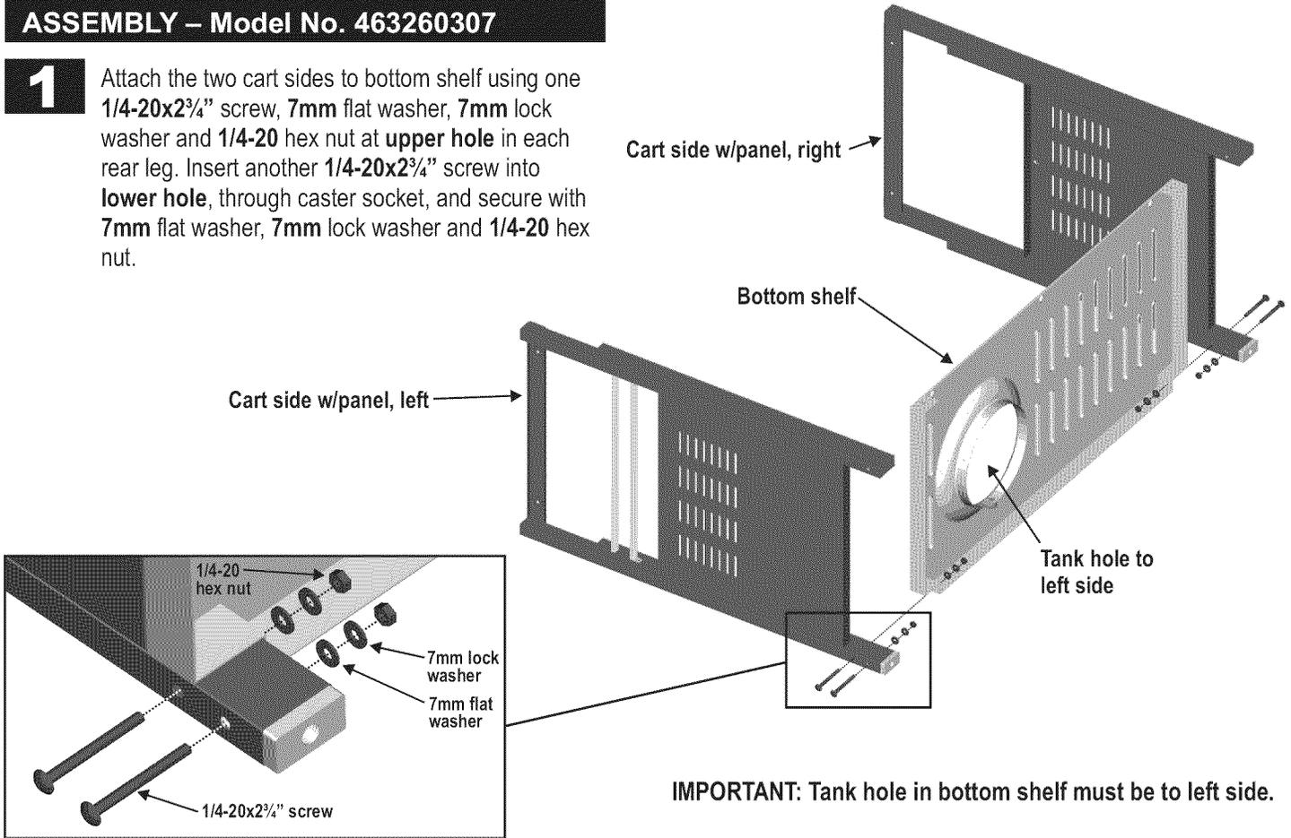
**IMPORTANT:** Tank hole in bottom shelf must be to left side.
