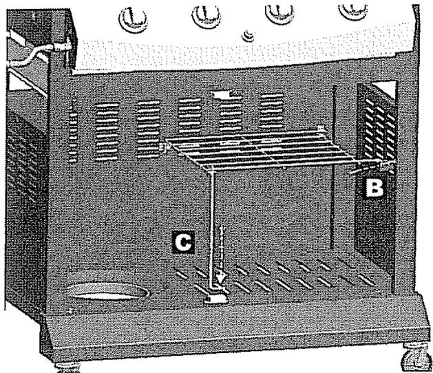
**15** Insert bottom door pin into hole in valance. Press the top door pin down, align with hole in door brace, release door pin. Repeat procedure on remaining door.
