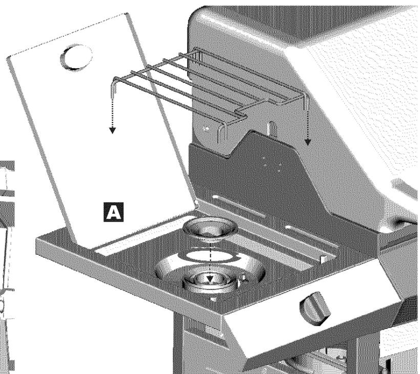
**11** Place flametamers (4) over burners by inserting tabs into slots in front of firebox. Opposite ends of flametamers rest on pins in back of firebox.
