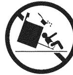
**⚠ WARNING** To reduce the risk of tipping, the range must be secured by properly installed anti-tip bracket(s) provided with the range. To check if the bracket(s) is installed properly, remove the lower panel or storage drawer and verify that the anti-tip bracket(s) is engaged. Refer to the Installation Instructions for proper anti-tip bracket(s) installation.
