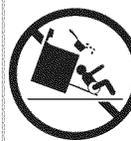
To reduce the risk of tipping, the appliance must be secured by properly installed anti-tip bracket provided with the unit. Refer to the Installation Instructions for proper anti-tip bracket installation.
