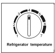
If you choose to change the thermostat setting, adjust the thermostat by one increment at a time. After each movement of the control knob, allow several hours for the unit to adjust completely. Large amounts of food may lower the cooling efficiency of the appliance.
