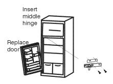
Place the refrigerator door on the bottom hinge. Ensure the door is aligned horizontally and vertically, and that the gasket seals on all sides before attaching the middle hinge. Attach the middle hinge using a screwdriver.
