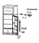
Remove the screws from the middle hinge. Lift the refrigerator door up and away from the appliance.
