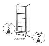
Remove the bottom hinge by removing the leveling leg and screws on the bottom of the refrigerator cabinet. To reattach the hinge on the opposite side of the cabinet, first remove the leveling leg. Reattach the hinge using the screws that were previously removed. Reattach both leveling legs.
