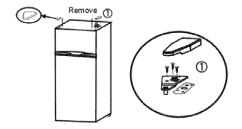
Remove the hinge cover. Unscrew and remove the top hinge.
