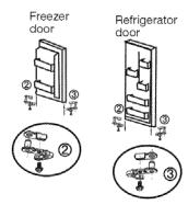
Remove the pin assembly from the bottom of the freezer and refrigerator doors. On the opposite side, attach the replacement pin assembly (located in the plastic bag with the Use and Care Manual) with a screwdriver. Note: You must re-use the screw from the pin assembly that is removed in this step when attaching the new assembly.
