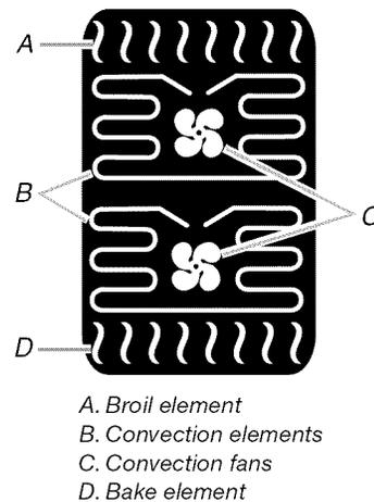
True Convect is best for baking 1, 2 or 3 racks of baked goods. During preheat the convect, bake and broil elements cycle to heat the oven. After preheat, only the convect elements and fans cycle on and off to maintain oven temperature.
