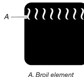
The element cycles on and off in intervals to maintain the oven temperature.
