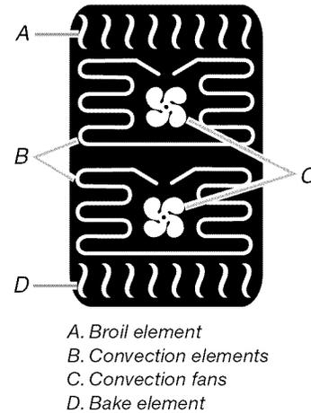
If the oven door is opened during convection roasting, the fans turn off immediately and turn on immediately when the door is closed. Bake, broil, and convect elements will turn off approximately 30 seconds after the door is opened. They will turn on again approximately 30 seconds after the door is closed.
