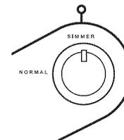
The simmer control knob has two settings: SIMMER and NORMAL. When the control is set on NORMAL, the left front surface cooking area or element will function as a single or dual element (on some models).
