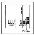
When you select a preset workout, the duration of the workout will appear in the upper display and a profile of the resistance levels of the workout will scroll across the center display
