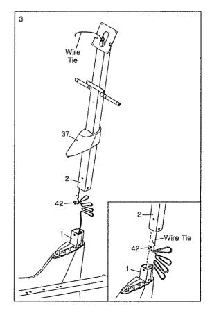
Slide the Upright (2) onto the Frame (1). Tip: Have a second person hold the Top Shield Cover (37) out of the way.
