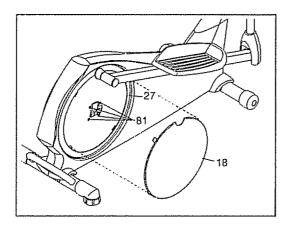
Then, remove the M8 x 14mm Button Screws (81) from the Right Pedal Disc (27), and gently rotate the Right Pedal Disc out of the way.
