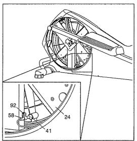
Next, rotate the Crank Assembly (24) until a Magnet (41) is aligned with the Reed Switch (58). Slide the Reed Switch slightly toward or away from the Magnet. Then, retighten the M4 x 16mm Screw (92).
