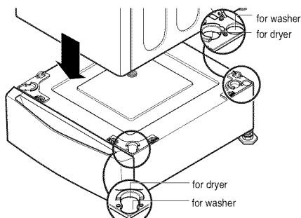
**NOTE:** The legs on the washer and dryer are not the same, so the recesses in the brackets on top of the pedestal are elongated. See the drawing above to identify the different locations for the washer and dryer legs. If the legs are not in the proper locations, the machine will not align properly and cannot be anchored to the pedestal.
