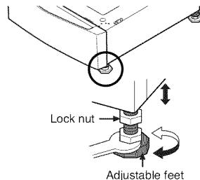
**NOTE:** Do not extend the legs no more than necessary to level the pedestal. The more the legs are extended, the more the machines will vibrate.
