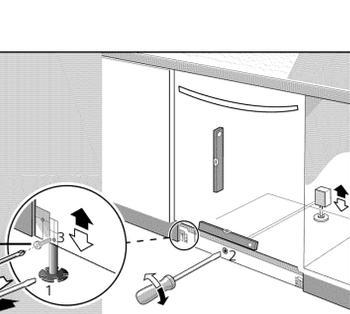
Level the dishwasher horizontally by turning feet (1) clockwise to raise or counter-clockwise to lower front of unit. Level vertically by turning center screw (2) to raise or lower the back. Once level, (3) insert leg leveler locking screws (part G) and tighten.
