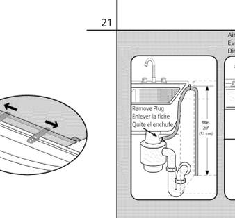
Note: Plumbing installations will vary - refer to local codes. Drain hose included is 92" (234 cm) and can be extended to a maximum of 150" (381 cm). Do not cut drain hose. Coil excess drain hose safely inside cabinet behind unit.
