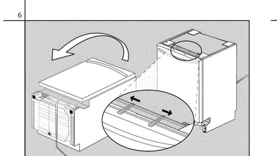
Flip unit back upright, ensuring water line remains in appropriate channel and is not pinched. If your dishwasher has the pre-attached mounting brackets shown and you have a wooden undercounter, ensure that brackets are positioned as far apart as possible by sliding them within slots in direction of arrows. Now skip ahead to step 9. Do not attach to countertop yet.
