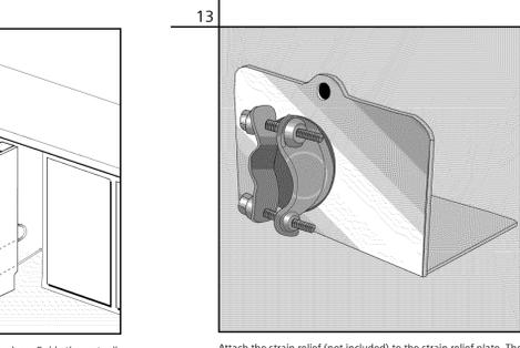
Attach the strain relief (not included) to the strain relief plate. The two screws on the back of the strain relief should be positioned as shown to prevent interference during assembly. Tighten the strain relief lock nut to prevent the strain relief from turning.
