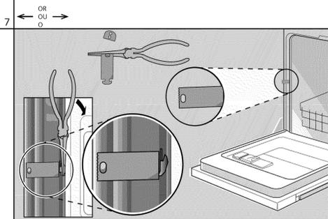
If your dishwasher has the pre-attached mounting brackets shown in figure 6, and the countertop is stone, using pliers, rotate the bracket flanges so that you are able to remove brackets from the top. Grasp bracket with pliers at perforation and bend until rounded end breaks free. Discard end. Slip brackets through side slots. Using pliers, bend bracket flanges such that the brackets will not slip through slots. Do not attach yet.
