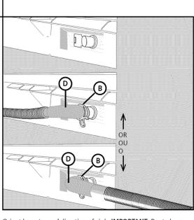
Orient hose toward direction of sink. **IMPORTANT:** Route hose toward sink PRIOR TO connection. Do not turn after attachment. Attach drain hose elbow (Part D) to back of unit with spring clamp (Part B). Do not use a power tool.
