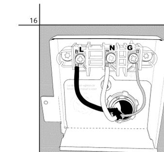
Note: Do not loosen or remove terminal screws! Damage may occur. Bend the wires so the exposed leads can reach the appropriate contacts. Insert the black (hot) wire into the left opening on the terminal strip marked "L", the white (neutral) wire in the middle opening of the terminal strip marked "N", and the bare copper or green (ground) wire into the right opening of the terminal strip marked "G".
