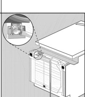
Attach hot water line to 90° elbow and route water line through channel as shown (stainless steel braided hose and PEX installations only - for copper consult a plumber).
