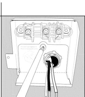
Place the assembled strain relief plate back into the junction box and re-attach the screw. Make sure the tab on the right side of the strain relief plate is outside the junction box as you slide it into place.
