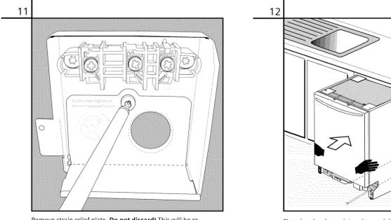
Remove strain relief plate. Do not discard! This will be re-installed later.
