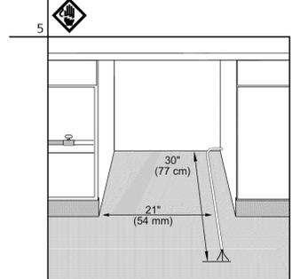
Turn power off at fuse box. Regardless of where the electrical supply cable originates, position it 21" (54 cm) from the opening's left side. Extend the cable 30" (77 cm) from the back wall.
