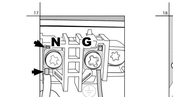
Make sure that the exposed (non-insulated) portion of each striped wire shows above and below the terminal screw. Securely tighten the terminal screws, but do not over-tighten or damage may occur.
