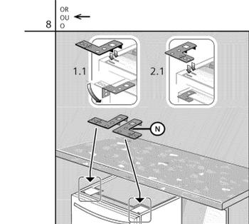
If your dishwasher does NOT have pre-attached mounting brackets shown in figure 7, attach the mounting brackets (part N) to the top of unit as shown in (1.1) for stone and in (2.1) for wooden undercounter. Do not attach to countertop yet.
