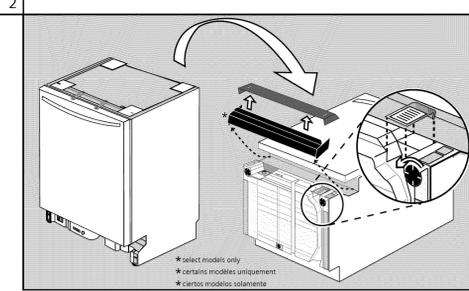
Gently rest the unit on its back. Remove the toe panels). Loosen front leg levelers slightly. Pre-adjust legs to approximate cabinet height. (See also step 19 for additional leveling instruction.) Remove junction box cover and retain for later use.
