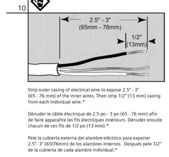
Strip outer casing of electrical wire to expose 2.5" - 3" (65 - 76 mm) of the inner wires. Then strip 1/2" (13 mm) casing from each individual wire.\*
