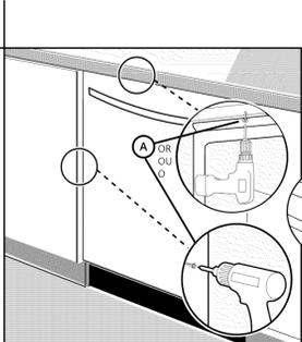
Prior to attachment, for top mount ensure that brackets are positioned as far apart as possible by sliding them within slots in direction of arrows. Insert screws (part A) through pre-positioned mounting brackets and attach unit to enclosure (pre-drilling of holes recommended).
