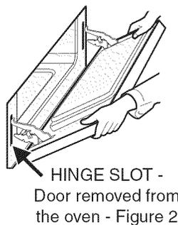
HINGE SLOT - Door removed from the oven - Figure 2
