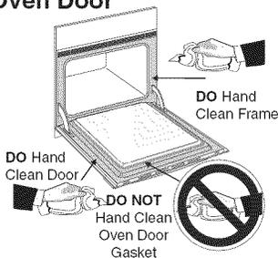
Use soap & water to thoroughly clean the top, sides and front of the oven door. Rinse well. You may use a glass cleaner on the outside glass of the oven door. **DO NOT** immerse the door in water. **DO NOT spray or allow water or the glass cleaner to enter the door vents.**
