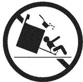
To reduce the risk of tipping, the appliance must be secured by properly installed anti-tip bracket provided with the appliance. To check if the bracket is installed properly; grasp the top rear of the appliance and carefully attempt to tilt it forward.
