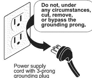
Power supply cord with 3-prong grounding plug
