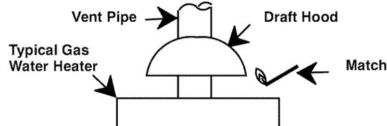
**NOTE:** If flame pulls towards draft hood, this indicates sufficient infiltration air.
