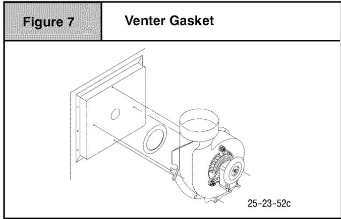
4. Replace venter gasket (part # 1013540, if needed) to venter assembly with adhesive in the same location as the old one.
