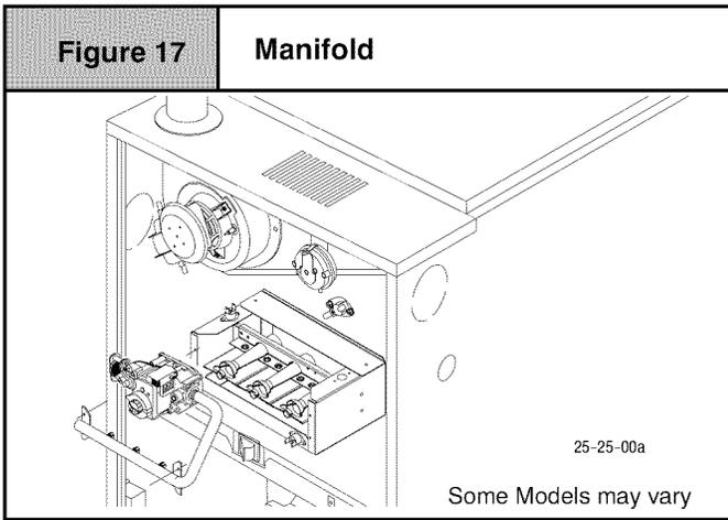
5. Carefully remove the manifold assembly.
