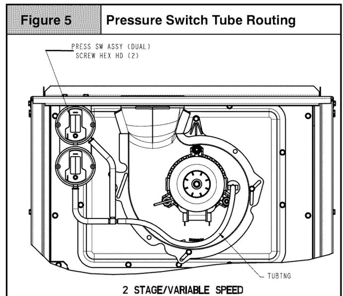
Note: When drilling new holes make sure metal shavings do not fall on or in components, as this can shorten the life of the furnace.
