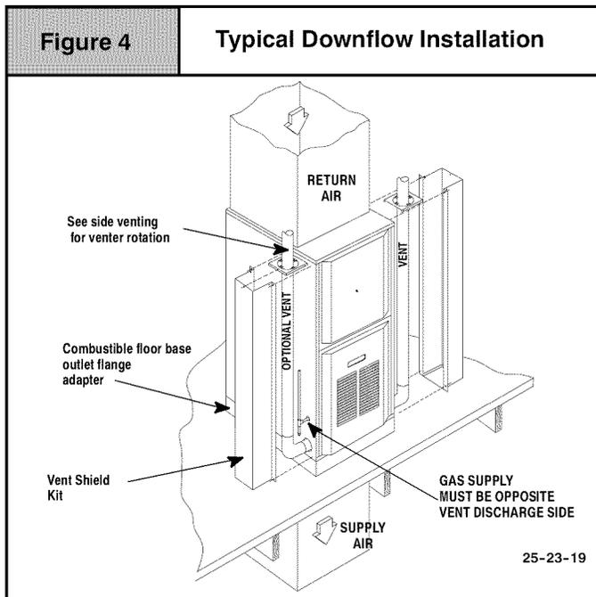
**Downflow Venting:** The combustion venter **MUST** be rotated to vent out the side for all downflow installations, (see **Figure 4**). Bottom venting is not permitted. See “**Side venting**” for instructions to rotate the vent to the side. In addition to rotating the vent to the side, a **Vent Pipe Shield** (NAHA002VC) is required to shield the hot vent pipe.
