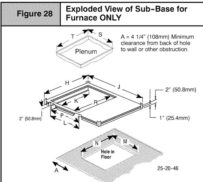
**Sub-base for Combustible Floors- Downflow Coil Adapter Box**
