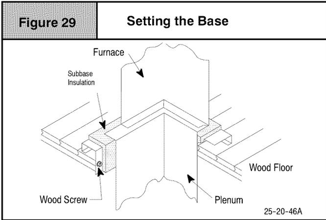
2. Fabricate the plenum to the dimensions given in **Table 7**. Note that the dimensions given are outside dimensions.
