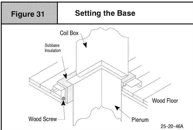
Consideration must be given to the height of the base to allow for easy installation of the condensate drain. See **Figure 32**. This subbase for combustible floors has been designed so that the
