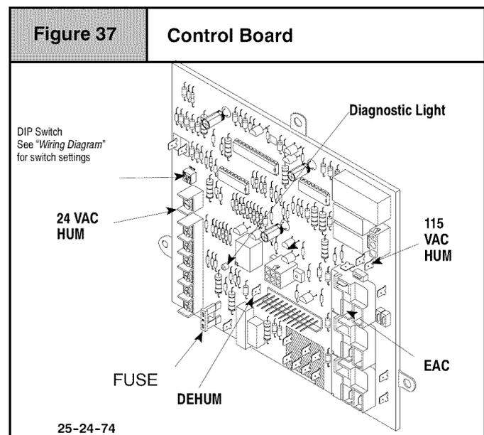
**HUMIDIFIER** - The 24VAC HUM is energized when the low pressure switch closes on a call for heat. The 115V HUM (called HUM on Control) is energized when the inducer is energized.
