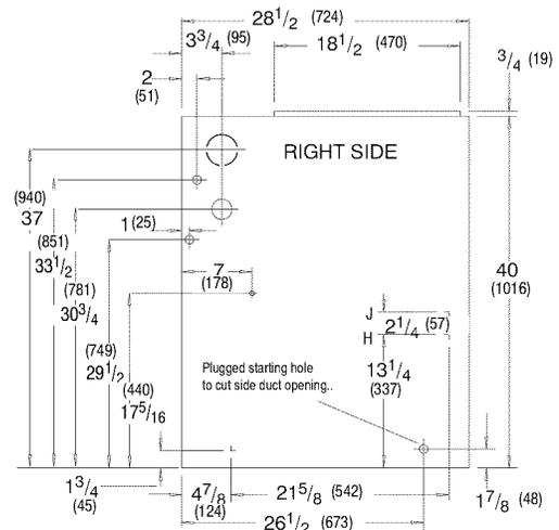
NOTE: Evaporator "A" coil drain pan dimensions may vary from furnace duct opening size. Always consult evaporator specifications for duct size requirements.
