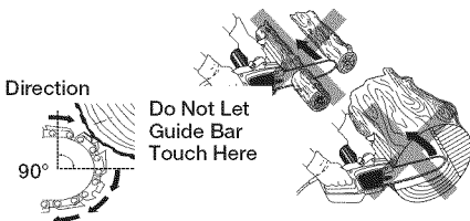
Figure 1 - Kickback Hazard Example: Do Not Let Nose of Guide Bar Touch Object While Chain is Moving
