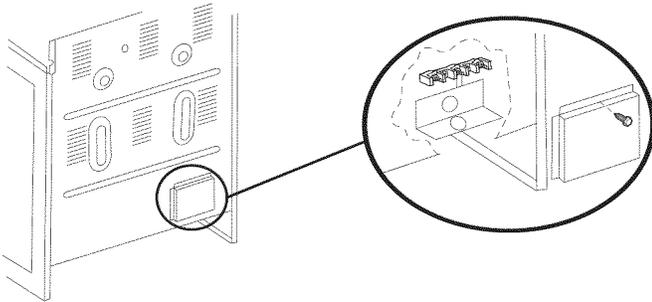
3. Remove plastic tag holding three 10-32 hex nuts from the middle post of the terminal block.
