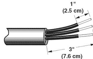
2. Allow enough slack in the wire to easily attach the wiring terminal block.
