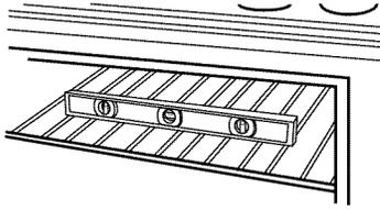
3. If range is not level, pull range forward until rear leveling leg is removed from the anti-tip bracket.
