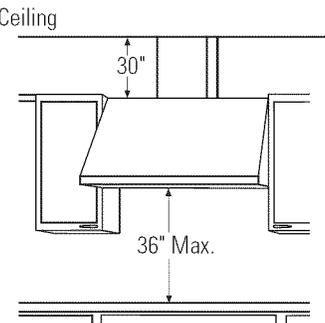
**10 ft. Ceilings:** Install the hood 32" min. to 36" max. above the cooking surface. The duct cover will expand to a maximum of 34" above the top of the hood to meet the ceiling.
