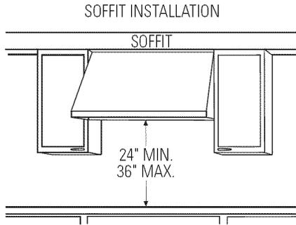
In this installation the ductwork running from the top of the hood will be concealed in the soffit or upper cabinetry.
