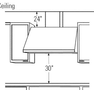
**9 ft. Ceilings:** Install the hood 24" min. and up to a maximum of 30" above the cooking surface. The duct cover will expand to reach ceiling height.
