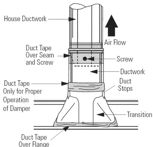
**CAUTION:** Do not use sheet metal screws at the transition to ductwork connection. Doing so will prevent proper damper operations. Seal connection with tape only.
