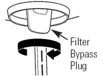
The bypass plug and the mini-manual are located in the top machine compartment.
