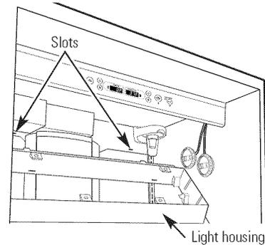
8. Holding up the light housing, place each lamp assembly in its holder. Feed the attached wires through the slots and tuck the wires outside the side of the light housing.
