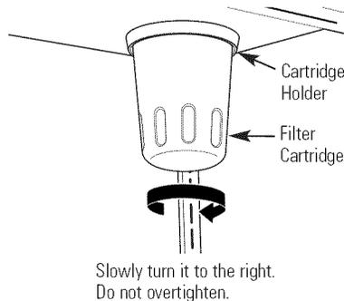
**IMPORTANT NOTE:** Remove the water filter to immediately stop any water leak from the Icemaker/Dispenser system. The water filter cartridge holder (bracket) acts as a cut-off valve when the filter is removed and will prevent further leaking.
