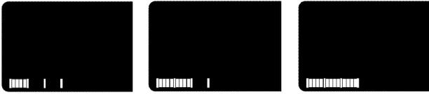
The progress bar is a visual picture of the estimated running time of a cooking cycle. It will appear during all cook cycles except Warm Hold. The lines in each of the segments will light from left to right as the time nears the end. When all 15 lines (all 3 segments) are lit, the cooking cycle is completed.
