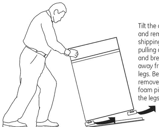
Tilt the dryer sideways and remove the foam shipping pads by pulling at the sides and breaking them away from the dryer legs. Be sure to remove all of the foam pieces around the legs.
