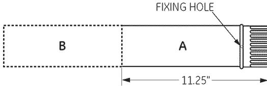
Cut the duct as shown and keep portion A.
