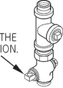
DISCONNECT AND DISCARD OLD FLEXIBLE GAS CONNECTOR AND OLD DUCTING MATERIAL. REPLACE WITH NEW CSA(AGA) APPROVED FLEXIBLE GAS LINE CONNECTOR AND UL APPROVED TRANSITION DUCT.
