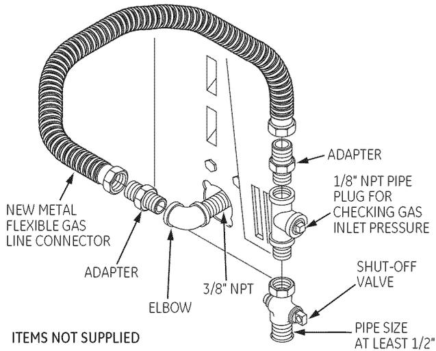
Note: The connector and fittings are designed for use only on the original installation and are not to be reused for another appliance or at another location. Keep flare end of adaptor free of grease, oil and thread sealant.
