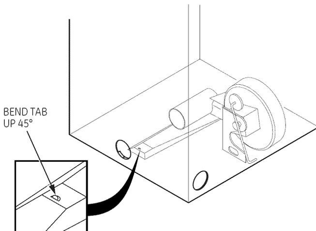
Through the rear opening, locate the tab in the middle of the appliance base. Lift the tab to about 45° using a flat blade screwdriver.
