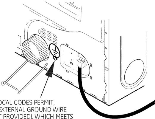
IF LOCAL CODES PERMIT, AN EXTERNAL GROUND WIRE (NOT PROVIDED), WHICH MEETS LOCAL CODES, MAY BE ADDED BY ATTACHING TO THE GREEN GROUND SCREW ON THE REAR OF THE DRYER, AND TO A GROUNDED METAL COLD WATER PIPE OR OTHER ESTABLISHED GROUND.
