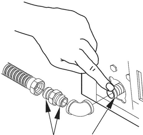
Tighten the flexible gas line using two adjustable wrenches.
