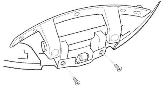
13. Hold the door on its side with one hand and fasten the remaining 2 screws as shown. Then tighten the 2 screws (#8) holding the hinge assembly.
