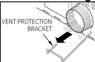
Pull the vent protection bracket out until it stops, and let it rest on the floor. The bracket prevents the unit from moving too close to the wall and crushing the rear vent.
