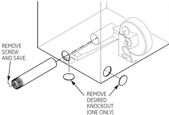
Detach and remove the bottom or left side knockout as desired. Remove the screw inside the dryer exhaust duct and save. Pull the duct out of the dryer. Protect sharp edges around the knockout and exhaust opening with the tape.
