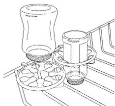
For best results, the Baby Bottle Holder should be installed on the upper rack of the dishwasher.
