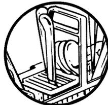
A cover can be lowered to either side to secure lightweight items from the effects of the vigorous wash action.
