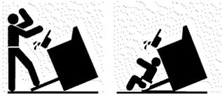
**⚠ WARNING:** If your range is removed for cleaning, servicing or any reason, be sure the anti-tip device is re-engaged properly when the range
