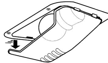
3. Replace the light bulb with an appliance bulb of the same wattage.
