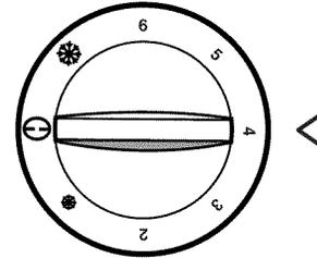
**NOTE:** To turn your refrigerator off, turn the refrigerator control to the setting shown. Your product will not cool when the refrigerator control is set to the off position.
