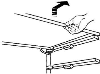
2. Replace the shelf by lowering the shelf stops through the openings in the refrigerator compartment liner. Slide the shelf in the rest of the way.
