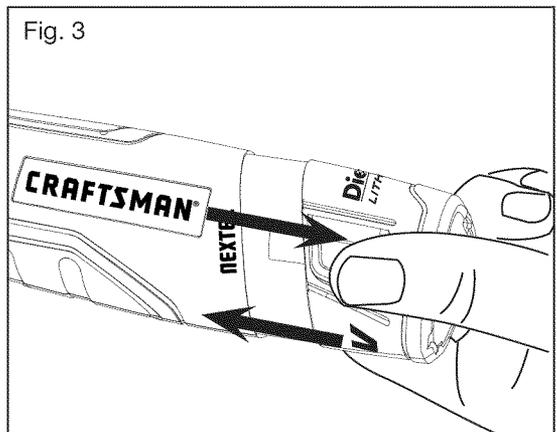
2. Make sure that the latch on the battery pack snaps into place and the battery pack is secured to the tool before beginning operation.
