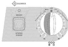
The ACCUSIMMER® Feature has two settings: SIMMER and NORMAL BURNER. When the switch is set on NORMAL BURNER, the left front surface cooking area or element will function as a single or dual element (on some models).
