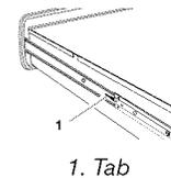
3. Press the tab down on the right side, and lift tab up on the left side at the same time, then pull drawer out another inch.
