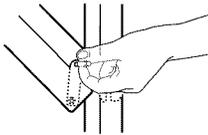
2. Carefully close the door until it rests against the door removal pins.
