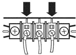
2. Place the hooked end of the neutral wire (white or center wire) of direct wire cable under the center screw of terminal block (hook facing right). Squeeze hooked end together. Tighten screw.
