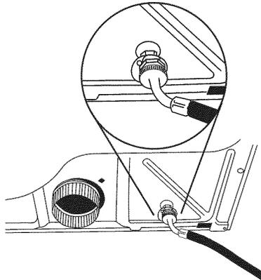
10. Using pliers, tighten the coupling an additional two-thirds turn.
