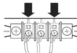
4. Tighten strain relief screw.
