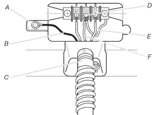
A. External ground conductor screw
