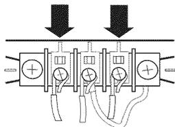
4. Tighten strain relief screws.
