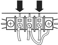
5. Tighten strain relief screws.
