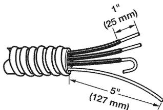
When connecting to the terminal block, place the hooked end of the wire under the screw of the terminal block (hook facing right), squeeze hooked end together and tighten screw, as shown.
