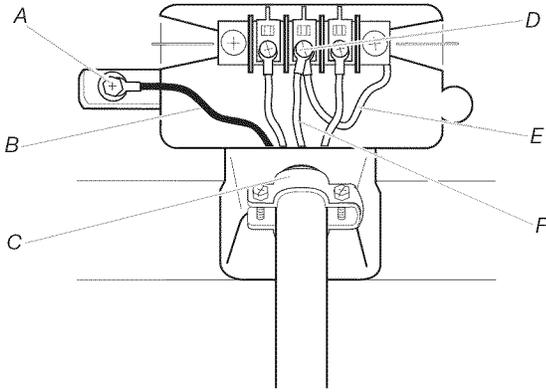
A. External ground conductor screw
