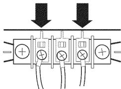
4. Tighten strain relief screws.
