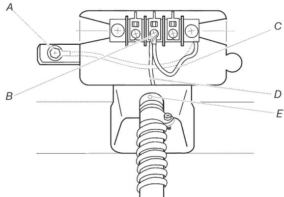
A. External ground conductor screw - Dotted line shows position of NEUTRAL ground wire before being moved to center, silver-colored terminal block screw.
