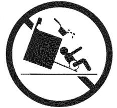
To reduce the risk of tipping, the range must be secured by properly installed anti-tip bracket provided with the range. To check if the bracket is installed properly, visually check that rear leveling leg is inserted into and fully secured by the anti-tip bracket by removing lower front panel or storage drawer from the range.
