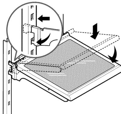
**CAUTION:** Make sure that shelves are level from one side to the other. Failure to do so may result in the shelf falling or spilling food.
