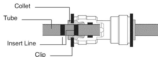
After inserting, pull the tube to make sure that it is secure and reinsert the clip.
