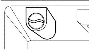
After changing the water filter cartridge, press and hold the Filter Reset button for 3 seconds; indicator light will go out.
