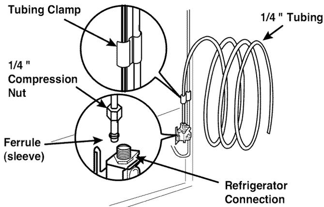
**▲ CAUTION:** Check to see if water dripping occurs at water line connections.
