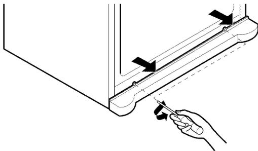
2. Turn the leveling leg clockwise to raise that side of the refrigerator or counterclockwise to lower it. It may take several turns of the leveling leg to adjust the tilt of the refrigerator.
