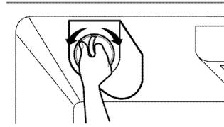
Push it in firmly until you can turn it. Using its handle, twist cartridge about 1/4 turn.
