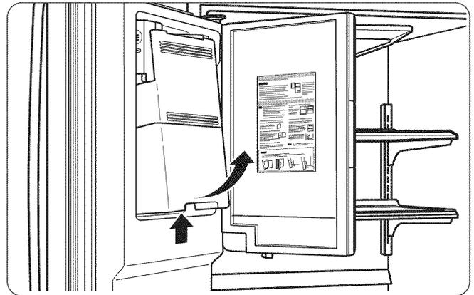
3. To reinstall the in-door ice bank, slightly slant the bin during replacement to avoid contact with the icemaker.
