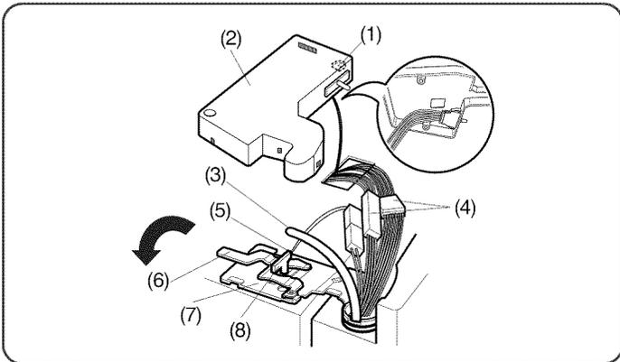
1. Open the door. Remove the top hinge cover screw (1).
