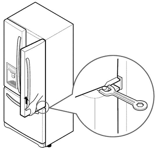
Level the refrigerator by using an 11/16 inch (18mm) wrench or a flat blade screw driver. Turn the leveling legs (CCW) to raise or (CW) to lower the height of the front of the refrigerator.
