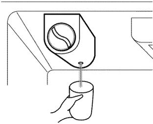
**NOTE:** When filter is being removed, the water drains through the hole.
