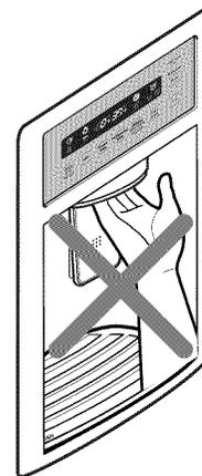
**▲ WARNING:** Do not put your fingers up the ice chute opening. Doing so can result in severe injury.
