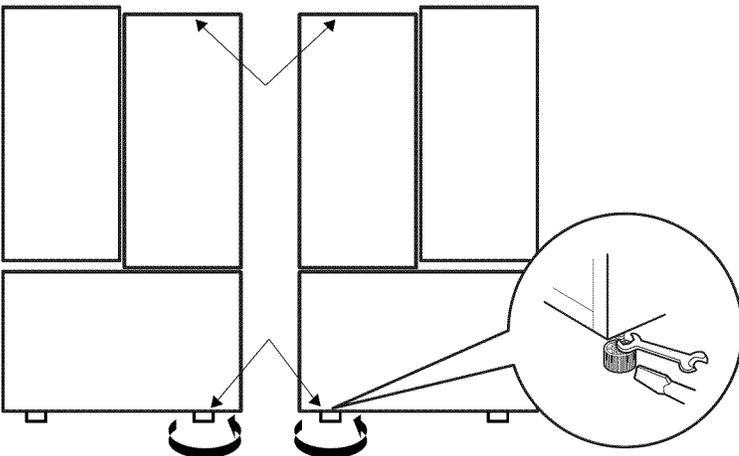
3. Open both doors again and check to make sure that they close easily. If not, tilt the refrigerator slightly more to the rear by turning both leveling legs clockwise. It may take several more turns, and you should turn both leveling legs the same amount.
