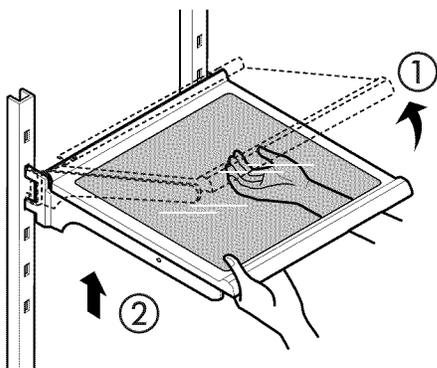
• **To reinstall a shelf**—Tilt the front of the shelf up and guide the shelf hooks into the slots at a desired height. Then lower the front of the shelf so that the hooks drop into the slots.
