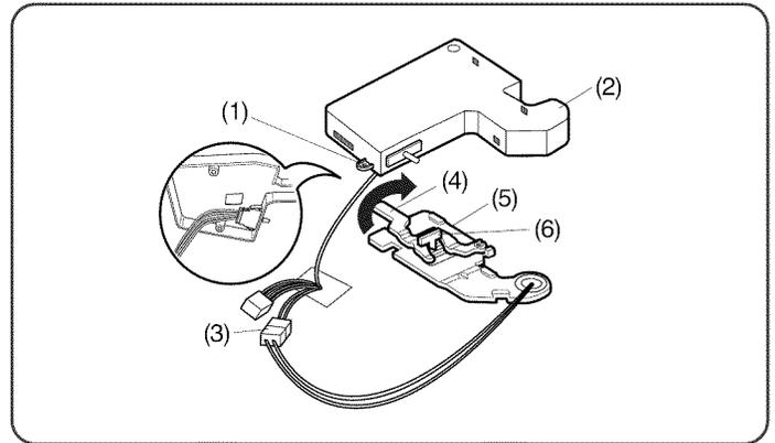
1. Open the door. Remove the top hinge cover screw (1). Lift up the cover (2).
