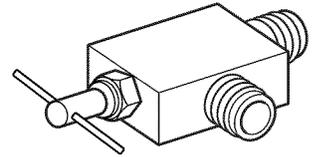
**NOTE:** Self Piercing Saddle Type Water Valve should not be used.
