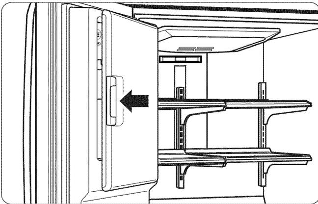
2. To remove the in-door ice bank, grip the front handle, slightly lift the lower part, and slowly pull out the bin as shown.
