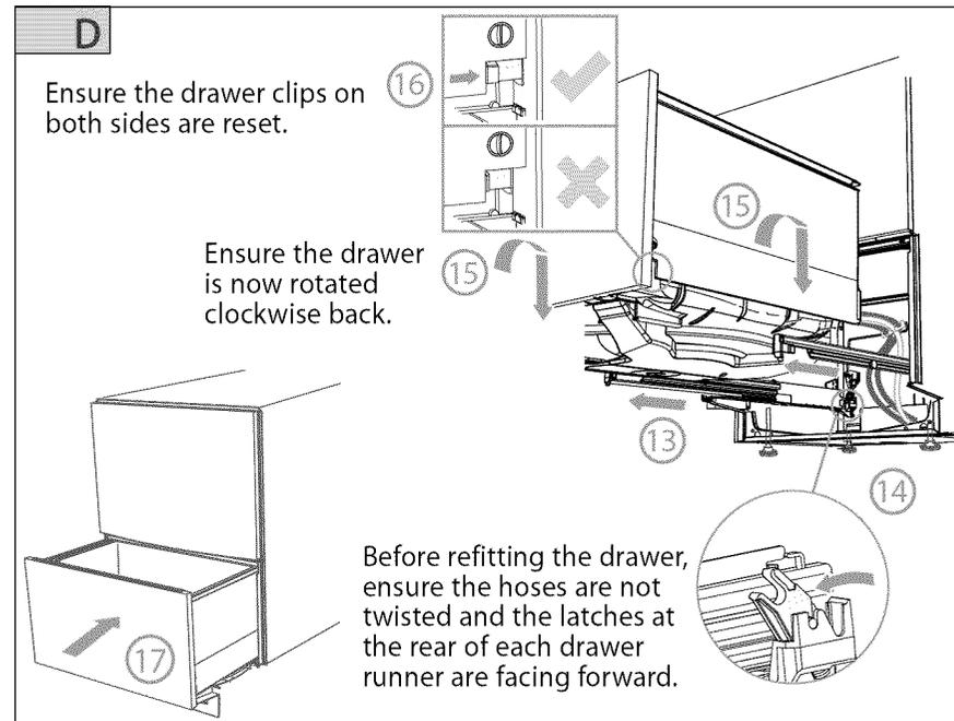
Ensure the drawer clips on both sides are reset.
