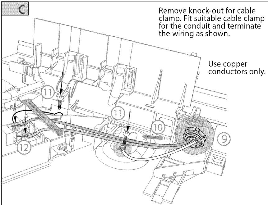
Remove knock-out for cable clamp. Fit suitable cable clamp for the conduit and terminate the wiring as shown.
