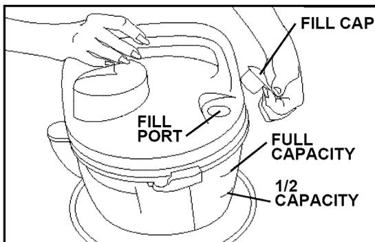
Remove fill cap. For a **full tank** of cleaning solution, pour **2 oz. of detergent** into tank through fill port and fill tank to "**full capacity**" line (1/2 gallon) with hot tap water.
