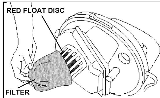
When the recovery tank is full, the automatic "shut-off" mechanism will turn off the cleaner suction.
