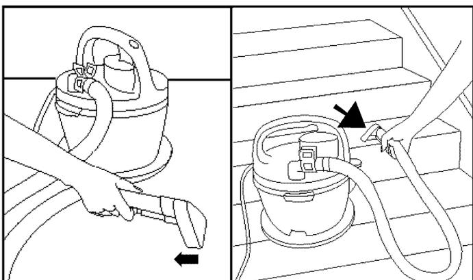
Lift nozzle, and position it at the edge of the carpet area or against the riser. Pull nozzle slowly over carpet without pressing trigger (dry stroke).
