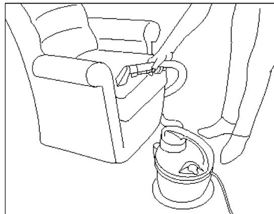
Gently press the nozzle onto the fabric. Press the trigger and slowly pull the nozzle over the fabric.
