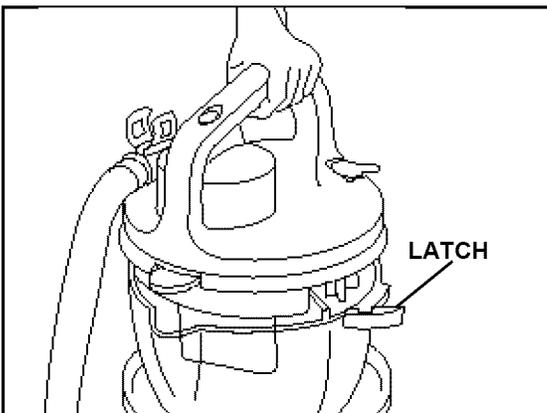
**c.** Unlatch cleaner lid by pulling latches outward on both sides of cleaner. Lift off lid.
