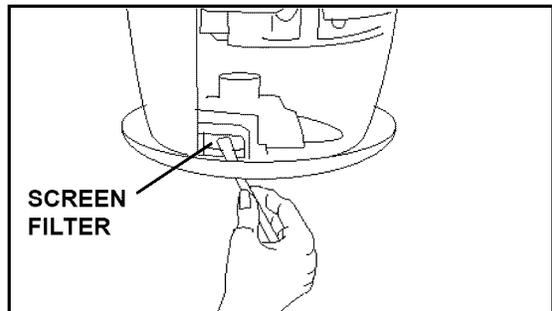
**f.** Remove debris from screen filter located at bottom of cleaner. Be careful not to poke through screen filter when cleaning.
