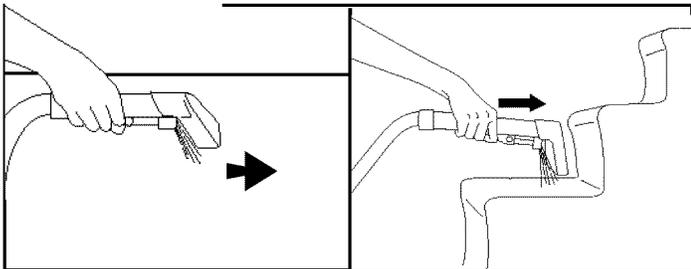
With cleaner placed on a stable surface, pre-spray a small area of carpet or carpeted stair by holding the nozzle about one inch above the carpet and push it forward while pressing the trigger (equals one wet stroke).
