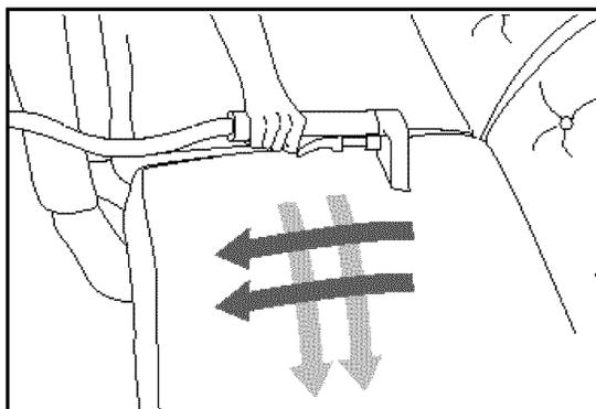
For heavily soiled areas, it may be necessary to repeat the cleaning process. Make crisscrossing strokes to the original pattern; overlap each pass.
