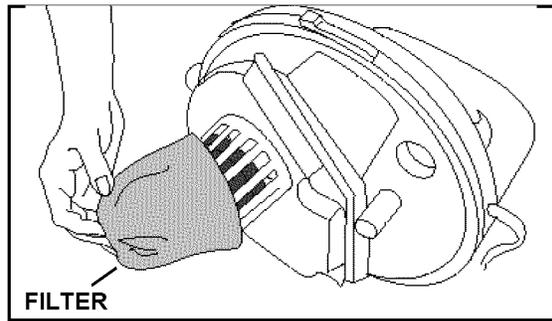
**d.** Remove debris from recovery tank filter and rinse with clean water. Filter may be removed for cleaning.
