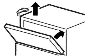
6.2.3. Make sure the door is slightly above the top of the cabinet and the gap between the doors is even across the front. Tighten the top hinge screws. Do not overtighten these screws—tighten them until they are just snug, then turn them another one-half turn.
