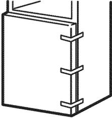
3.2 Using a 5/16" hex-head socket screwdriver and a 5/16" open-end wrench, remove the two screws holding the center hinge to the cabinet. Lift the center hinge to free its pin from the socket in the top of the door, and set hinge and screws aside. **Be careful not to lose the center hinge spacer and washer.**
