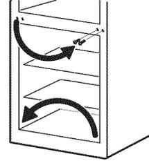
3.7 Take one of the screws removed in step 2 and start it in the outermost screw hole on the opposite side. Do not drive it all the way down—leave enough space under the screw head for thickness of the bracket.
