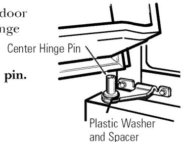
6.2.2 Tilt the door toward the cabinet, lifting the top hinge so the pin fits into the socket on the top of the door.
