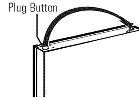
5.1.5 Pull the plug button from the front of the door and transfer it to the opposite side.
