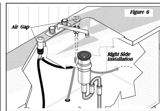
3. If you connect to a sink trap, local codes may require you to install an air gap kit, not included. The drain hose will be routed from dishwasher to air gap inlet as shown in Figure 6. An air gap kit is available from a plumbing supply store.
