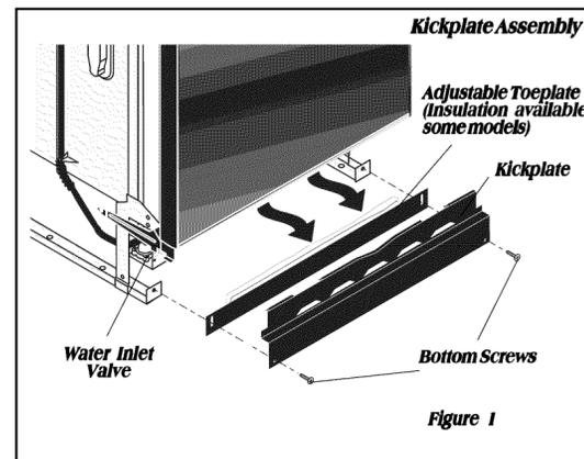
3. Locate water inlet valve behind kickplate on bottom left underside of unit. The valve has a  $\frac{3}{8}$ " NPT female fitting.
