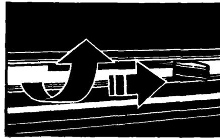
2. Lift the panel between the upper and lower oven doors. Move the Lock Lever all the way to the right.
