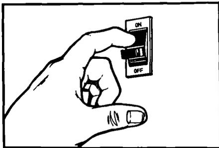
1. **WARNING:** To avoid possible shock hazard, turn off the electric power at the main power supply.
