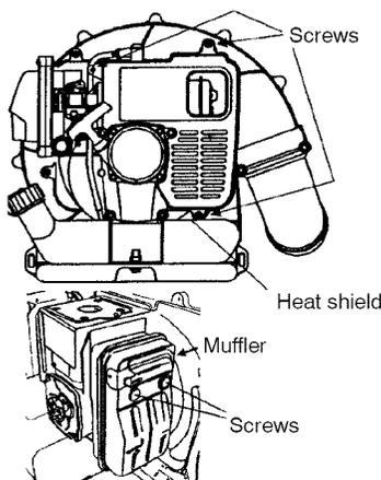
3. Remove the spark arresting screen.
