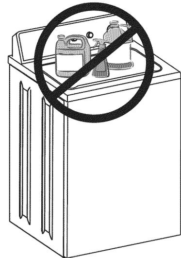
**IMPORTANT** Do not store or place laundry products on top of washer at any time. They can damage the finish or controls.
