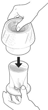
If a build-up of fabric softener occurs, clean with hot water. **DO NOT REMOVE SERVICE CAP FOUND INSIDE THE AGITATOR POST.**
