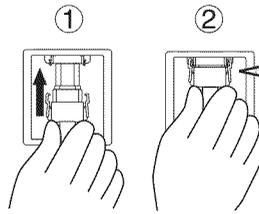
Insert it firmly until the tabs on both sides click into place.
