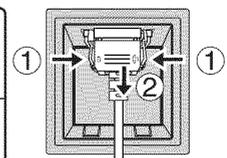
Press both tabs and pull the AC cord plug away from the TV.
